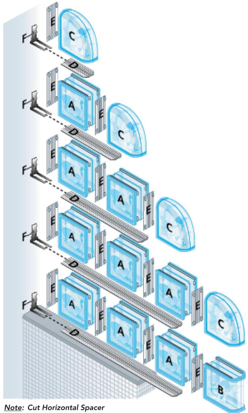
Note: Cut Horizontal Spacer to fit each row of blocks.
